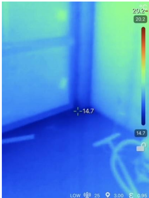
Window sill — cool zone at 14.7°C indicating active moisture ingress at the sill/frame junction
